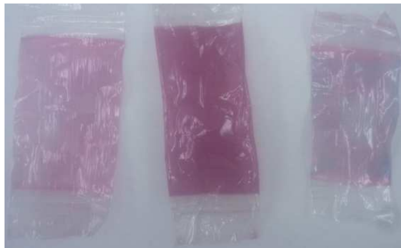
FIGURE 16 – Image of 8 (left), 12 (middle), and 15kDa (right) cellulose membranes in the presence of \text{HAuCl}_4
